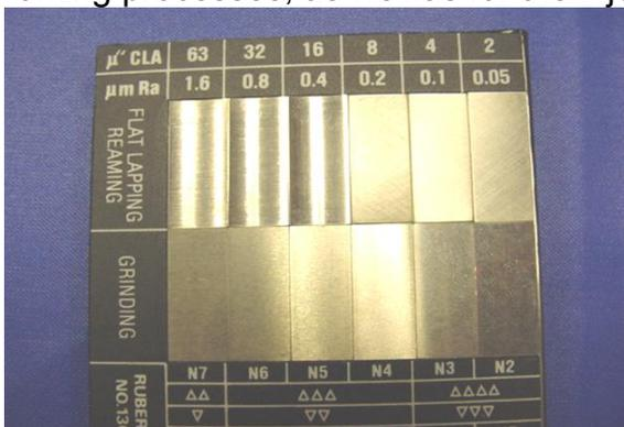
Fig.4. Roughness gauge for chipping worked surfaces.
