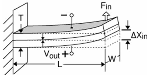
Fig.9. Principle of the piezoelectric sensing head.
