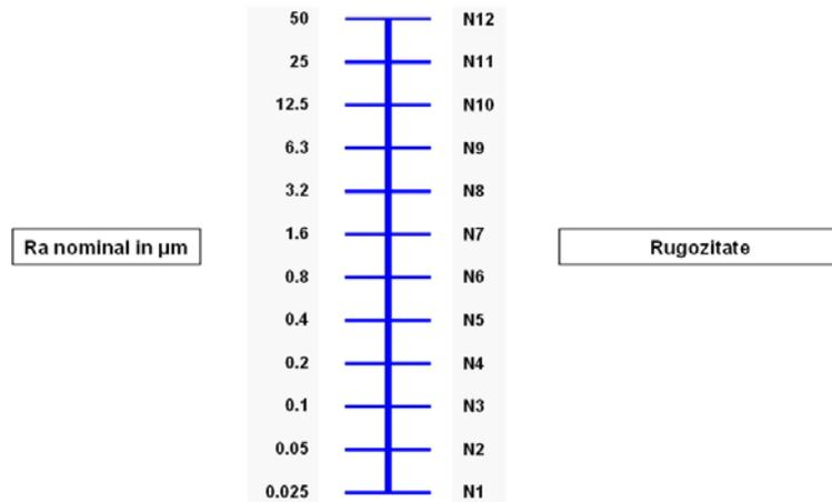
Fig.6. Correspondence between the nominal roughness Ra and the gauge worked surface.
