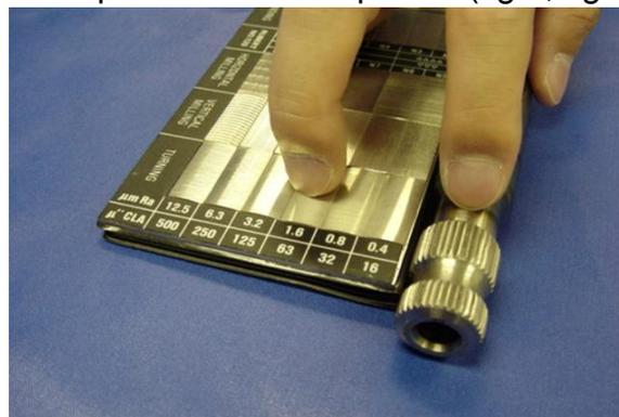
Fig.5. Checking of the surface quality of an axle by comparison and feeling.
