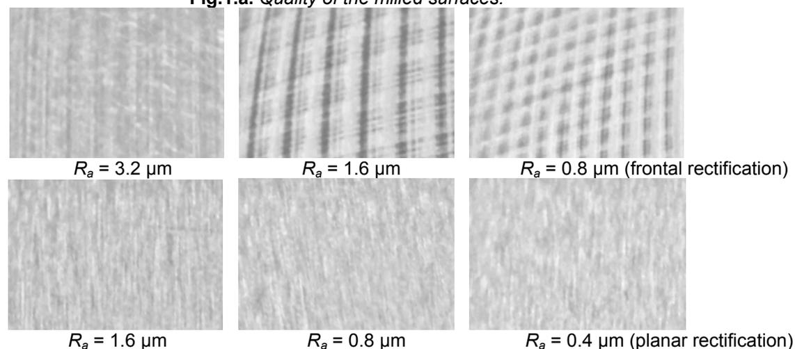
**Fig.1.b.** Quality of the rectified surfaces.
