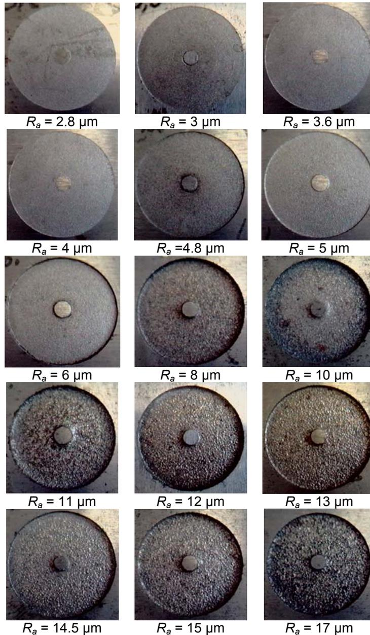
**Fig.14.** Frequently used roughness values for thermoplastic materials injection dies – magnified 10x on the CITIVAL microscope.
