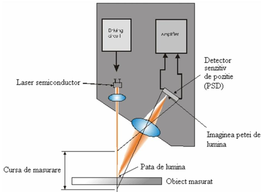
**Fig.13. Working principle of the contact-free laser instrument.**
