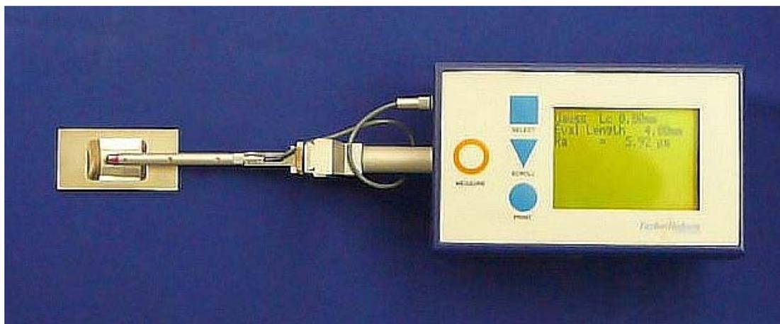
Fig.15. Calibration of the roughness meter.
