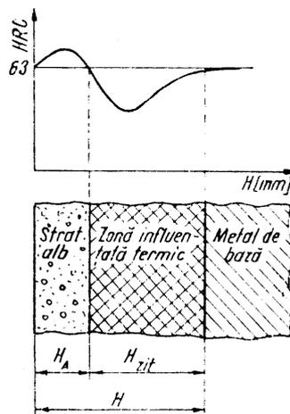
Fig.2. Superficial layer after electrical discharge working.
