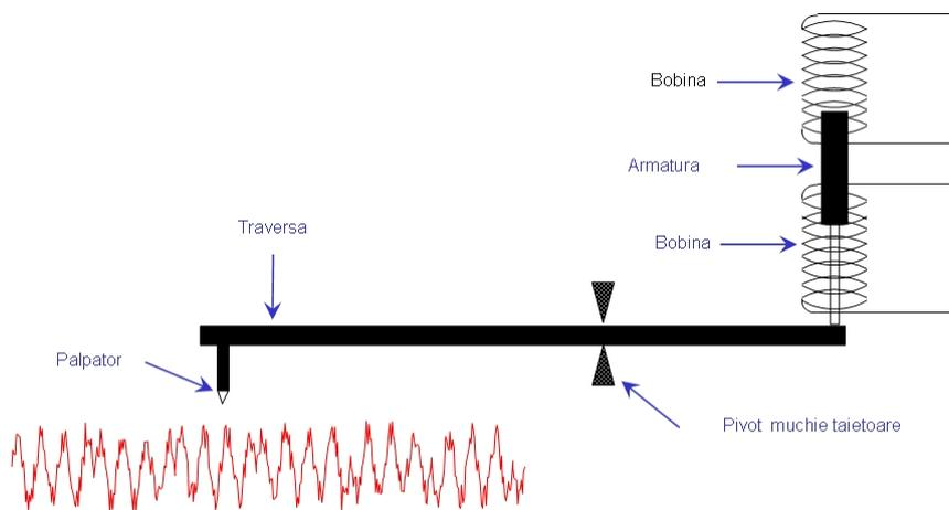
Fig.8. Principle of the inductive sensing head.
