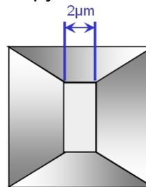
Fig.12. Truncated pyramid shaped pin.
