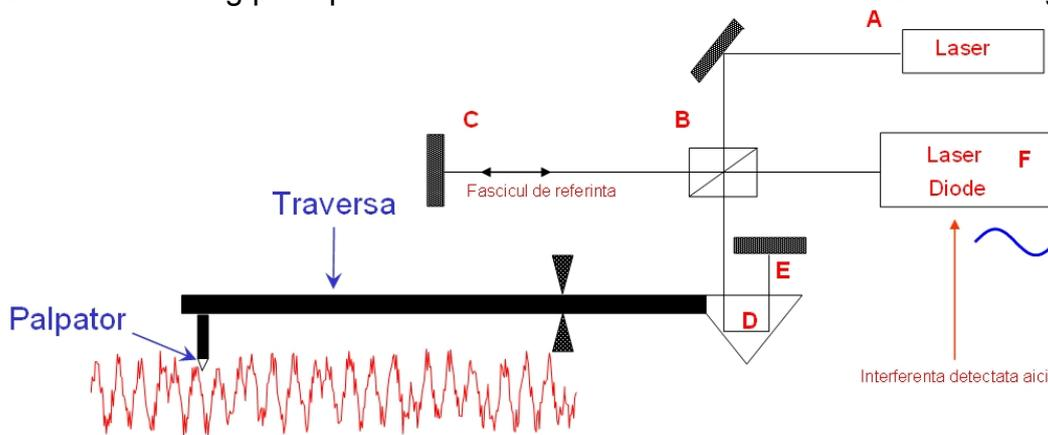
Fig.10. Laser interferometer sensing head.
