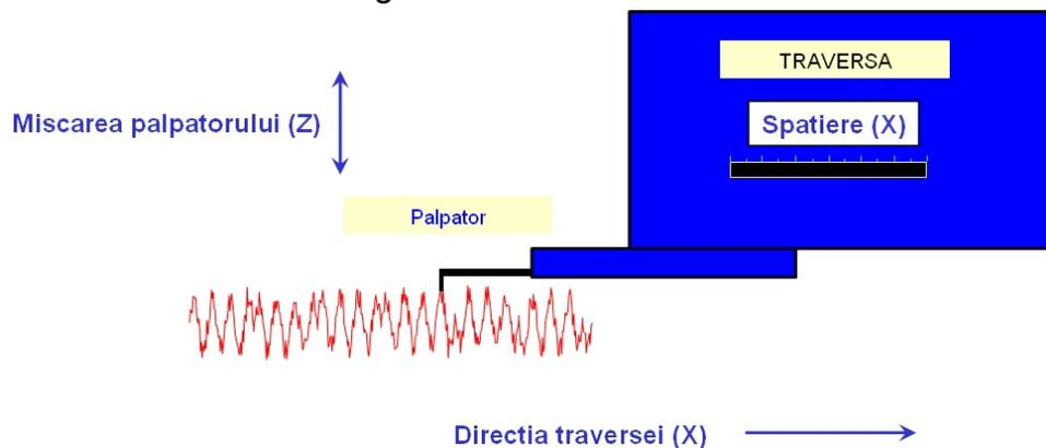
Fig.7. Principle of contact instruments.
